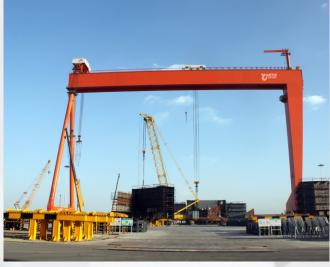
Rail-mounted shipyard gantry crane
